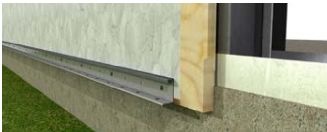
Vertical (Panel) Starter Track fastened every 8" to wood framing and sheathing
