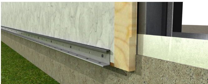
Vertical Starter Track fastened every 8"
