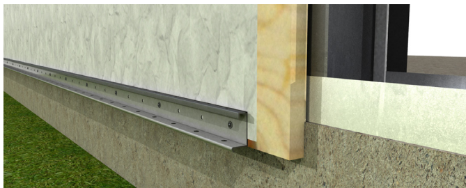
Vertical Starter Track fastened every 8"
