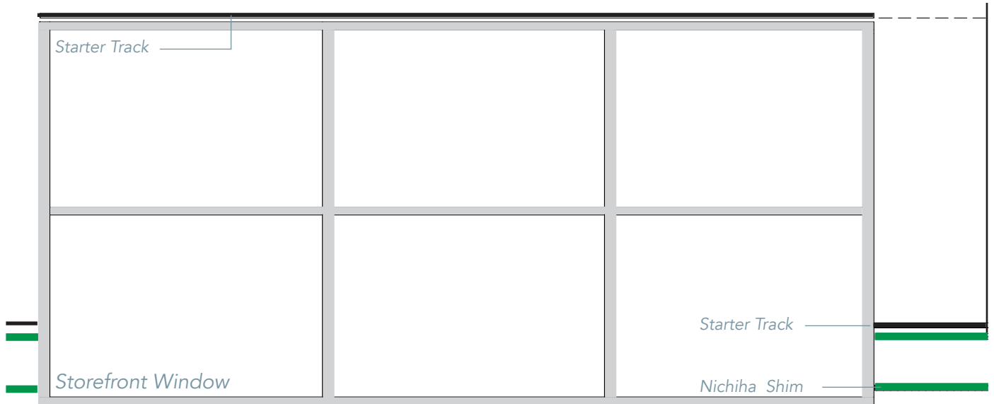
Make strategic use of Starter Track above and adjacent to large openings to course and align panel joints as desired.
