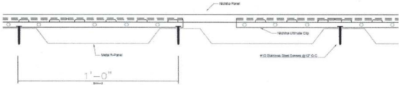
**Figure 5 - Typical Installation Over PEMB Metal R-Panel**
