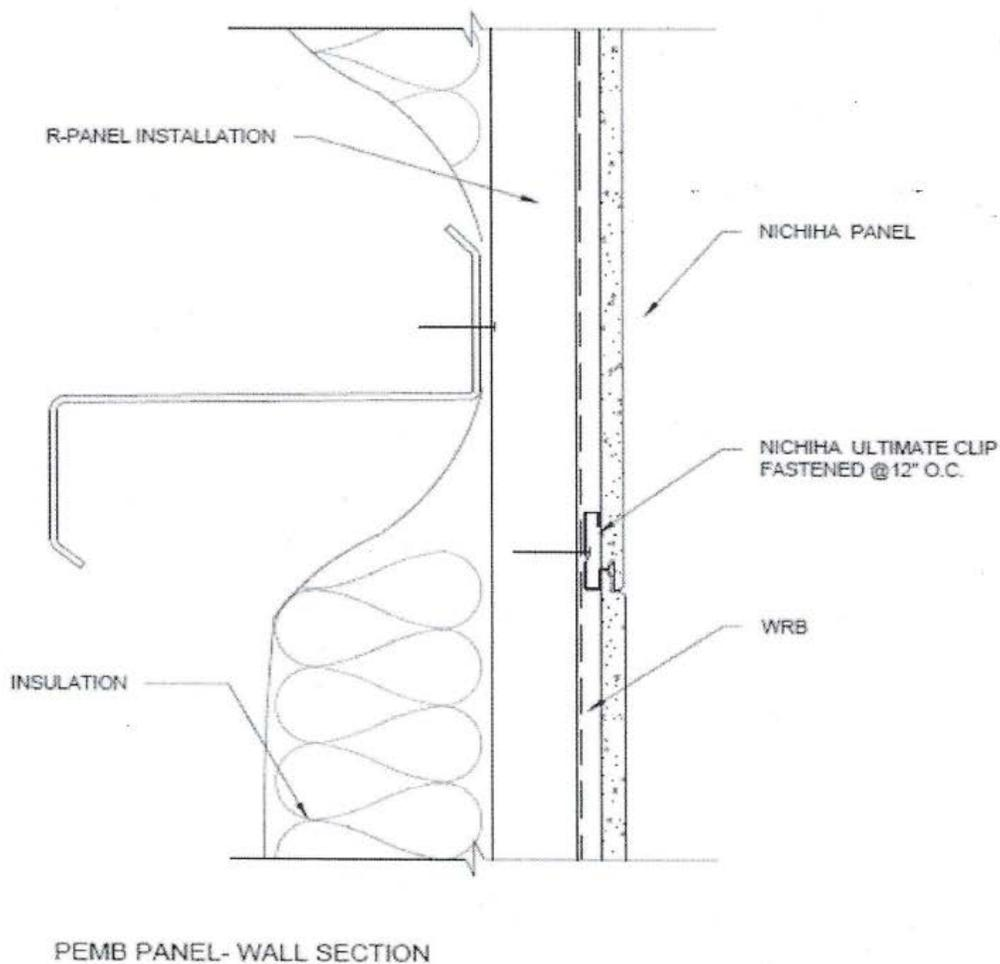
**Figure 6 - Typical PEMB Panel Wall Section**
