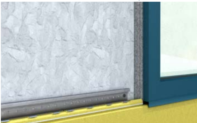
Flush window jamb with Sealant Backer
